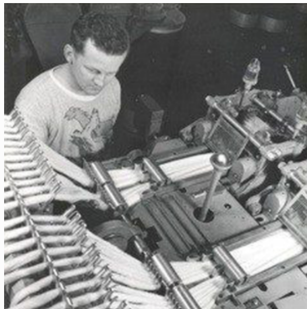
Carding machines produced a rope-like material called sliver. Roving machines refined the sliver, shown in this c. 1950 photo taken at the American Thread Company's Willimantic plant, into roving, a more regular product that could fit into a spinning frame. From the collections of the Windham Textile and History Museum.
