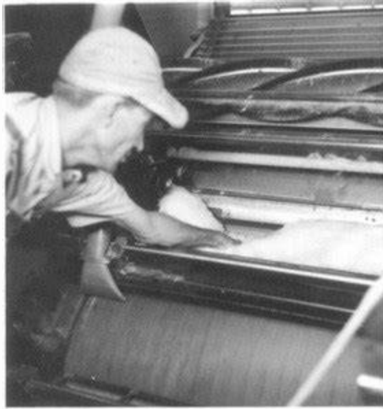
This staged 1943 photo was probably taken to accompany a safety brochure. It shows an American Thread Company employee pretending to put his hand into a carding machine. If this scene had been real, the worker would probably have lost his hand. From the collections of the Windham Textile and History Museum.
