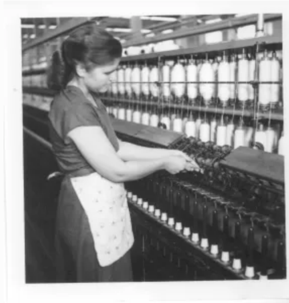
A worker tends a spinning frame, which stretched and twisted roving into thread. From the collections of the Windham Textile and History Museum.
